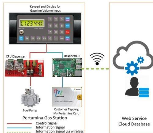
**Figure 5. Block Diagram of Proposed M-Payment System**
